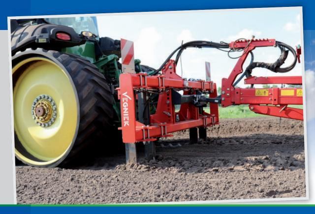
THE SUBSOILER WITH HYDRAULICALLY EXTENDABLE TINES
